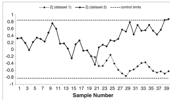
Figure 3. Graphical display of the  $S^2$ -EWMA chart with  $\lambda=0.2$  and  $L=2.592$
