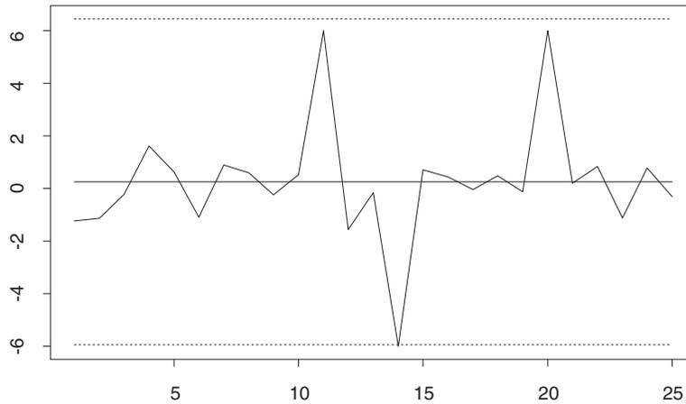
Figure 1. Control chart with control limits based on the average moving range.
