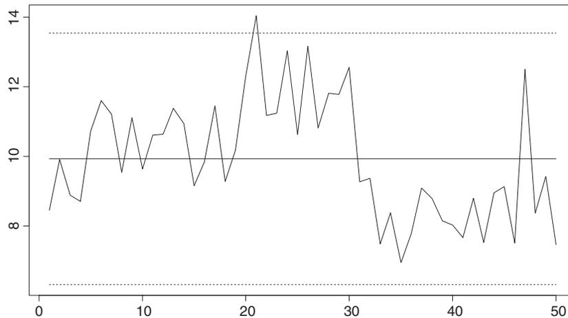
Figure 2. Control chart with control limits based on the average moving range.
