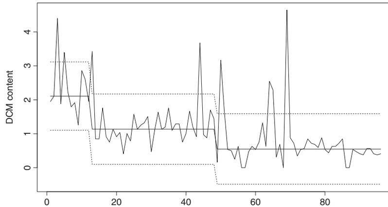
Figure 5. Proposed control chart for DCM percentage measurements.
