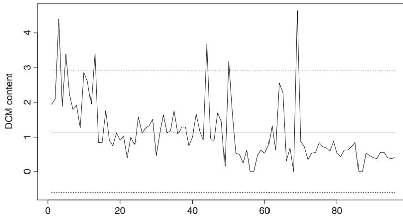
Figure 6. AMR chart for DCM percentage measurements.
